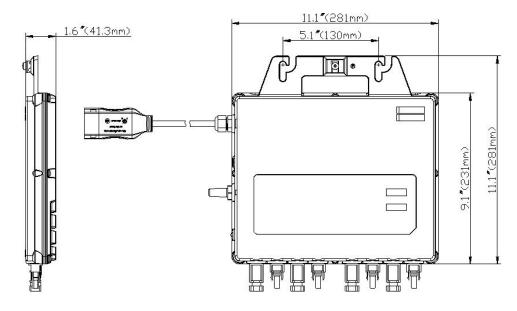
The APsystems QS1 is a grid-tied microinverter with intelligent networking and advanced monitoring systems to ensure maximum efficiency. High efficiency, high reliability of the QS1 with 4 independent MPPT inputs, Maximum AC output power reaching 1200W. Quarter the inverters and quarter the installation means real cost savings for residential and commercial customers.
